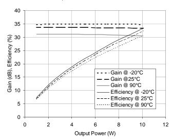
Gain and Efficiency vs. Output Power and Temperature Freq=950 MHz EDGE, Vdd=28 V
